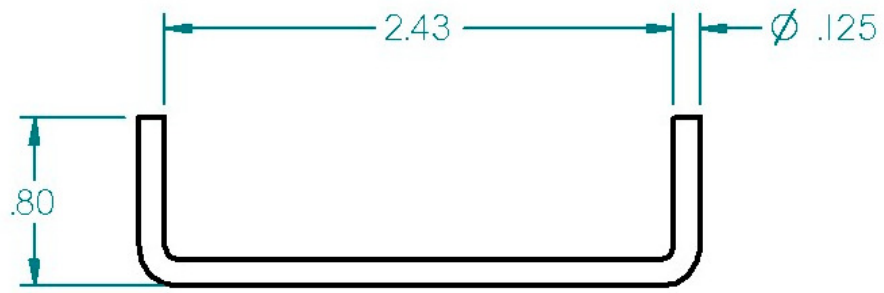
Figure 3. Clutch assembly wire dimensions. Not to scale.
